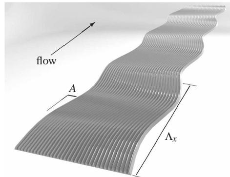
Figure 1: Schematic of meandering riblets.
