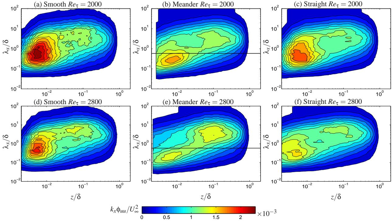
Figure 3: Premultiplied energy spectra  $k_x \phi_{uuu} / U_\infty^2$  contours for (a,d) smooth wall (b,e) meandering and (c,f) straight riblets at two Reynolds Number as indicated, plotted as a function of wall normal position  $z/\delta$  and energetic streamwise length scale  $\lambda_x/\delta$ .
