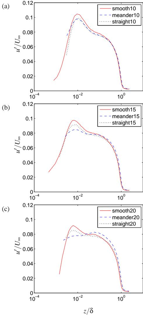
Figure 2: Freestream normalised RMS turbulence intensities  $u'/U_\infty$  for smooth wall, meandering and straight riblet surfaces at (a)  $Re_\tau = 1400$ , (b)  $Re_\tau = 2000$  and (c)  $Re_\tau = 2800$ .
